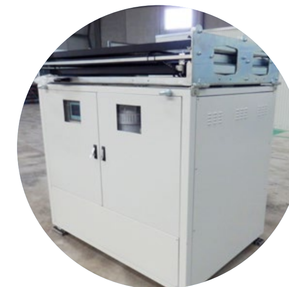
Mexico Aguascalientes Arsenic removal 1.5 m 3 /h (1 unit)
